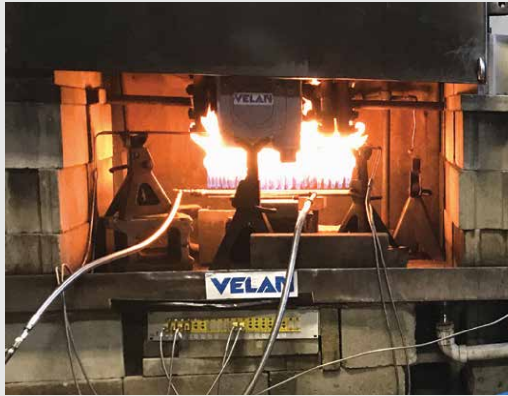
Duke Tran, witnessing the fire testing of five Velan valves including ball and triple-offset valves, resulting
