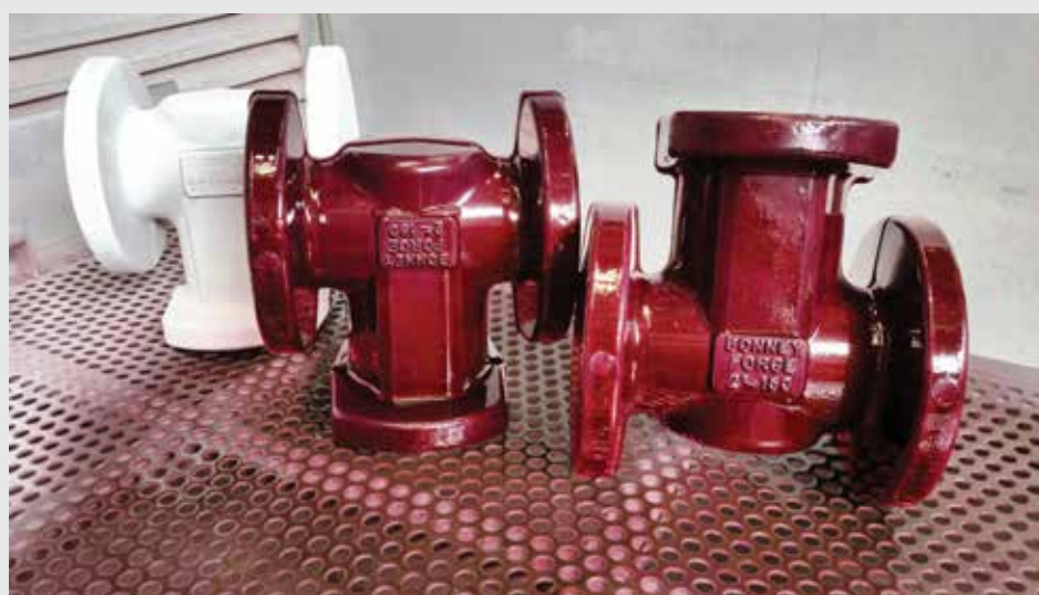
Pictured here are forged Alloy 825 gate valves undergoing in-house Dye Penetrant testing.
