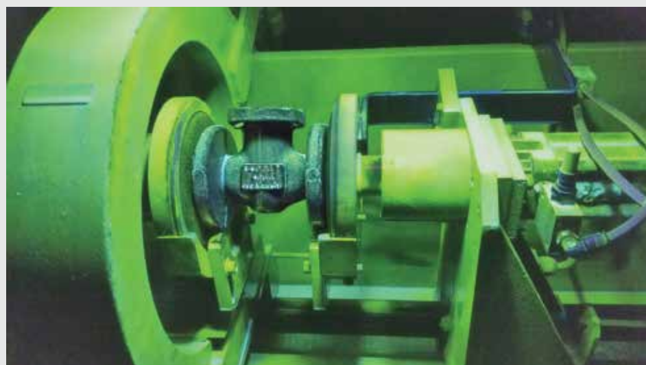
Pictured here valve bodies mounted in Bonney Forge's in-house magnetic particle test bench, this test utilizes a wet fluorescent liquid to detect flaws.
