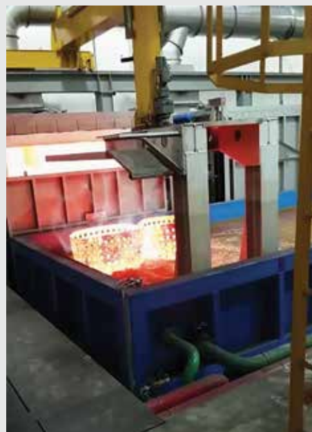
Shown here is the new, in-house, state of the art, automated heat treatment furnace and aerated quench tanks thermally stabilizing a fresh batch of F347 Stainless Steel forgings.
