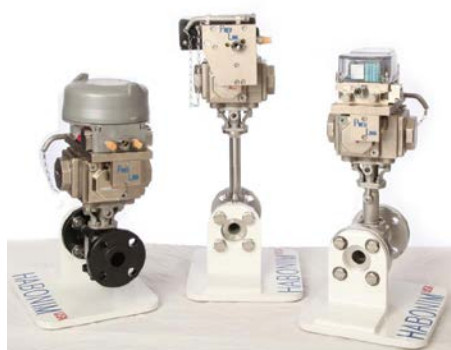
PNEU-LINK assemblies on various valves and accessories
