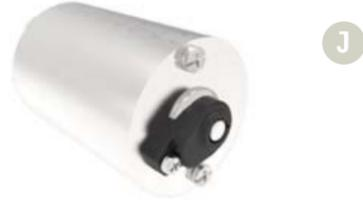
**J. Electromechanical Brake** - The electromechanical brake slows or stops the motor using electromagnetic force to apply mechanical resistance to the spindle. The electromechanical brake is also installed on the bottom of the motor shaft.
