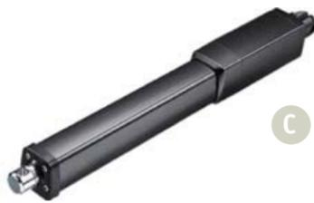
**C. Inline Actuators** - An inline actuator has a longer retracted length, but is designed specifically to fit into smaller or compact spaces. The inline actuator is typically made up of a motor, planetary gear assembly and drive spindle. These usually operate at a higher noise level.
