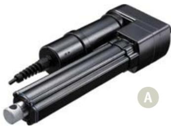
**A. Parallel Drive Actuator** - The motor is directly parallel to the drive spindle. Typically, these types of electric linear actuators are spur gear or belt driven with more gear ratio options. Parallel drive actuators allow for a wider range of loads and speeds; however, they can operate louder than worm gear driven actuators.
