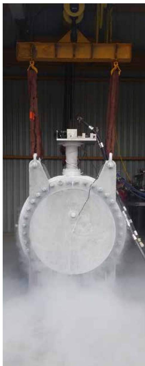
BS&B facilities for cryogenic testing of valves in liquid nitrogen at -324°F
