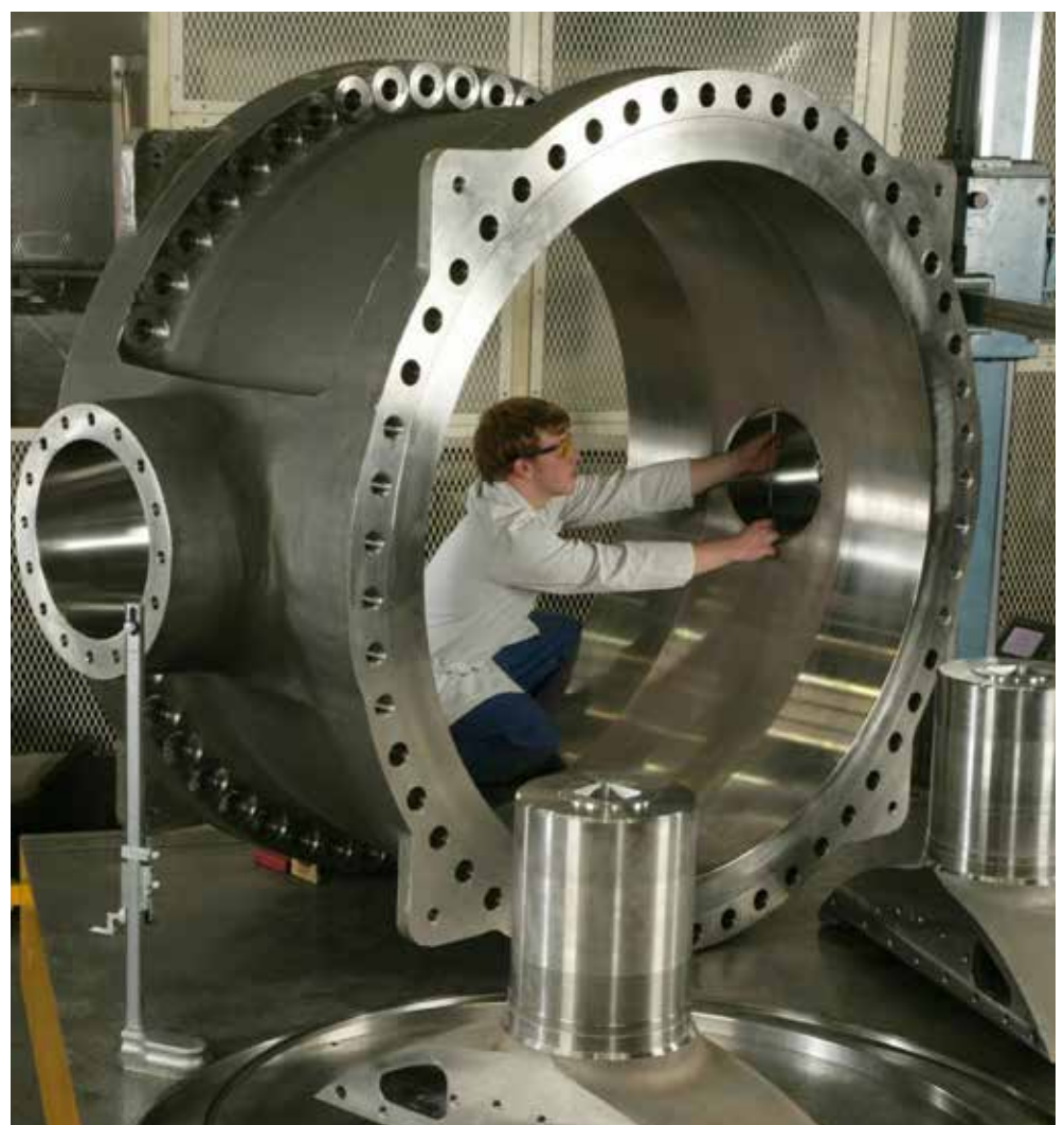
The largest ASME certified Bucking Pin Device in the world - 60" BPRV
