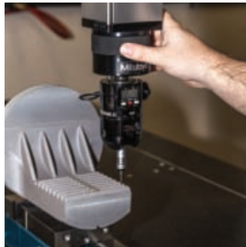
The CMM machine, above, lets UniTorq confirm the consistency of parts accurately and is one of several machines used to raise standards and assure higher quality.
