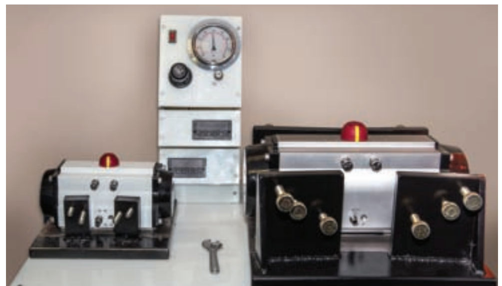
UniTorq has developed a test bench capable of determining torque beyond theoretical values. This allows them to back up their product claims with actual torque measurements.
