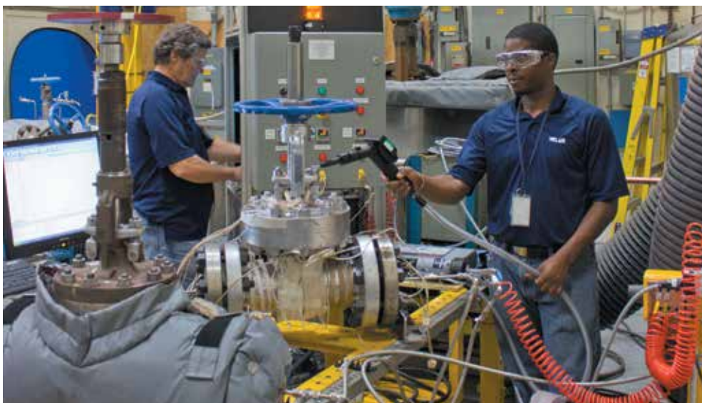
Fugitive emissions testing of a 4" (100 mm) Class 600 cast steel gate valve.
