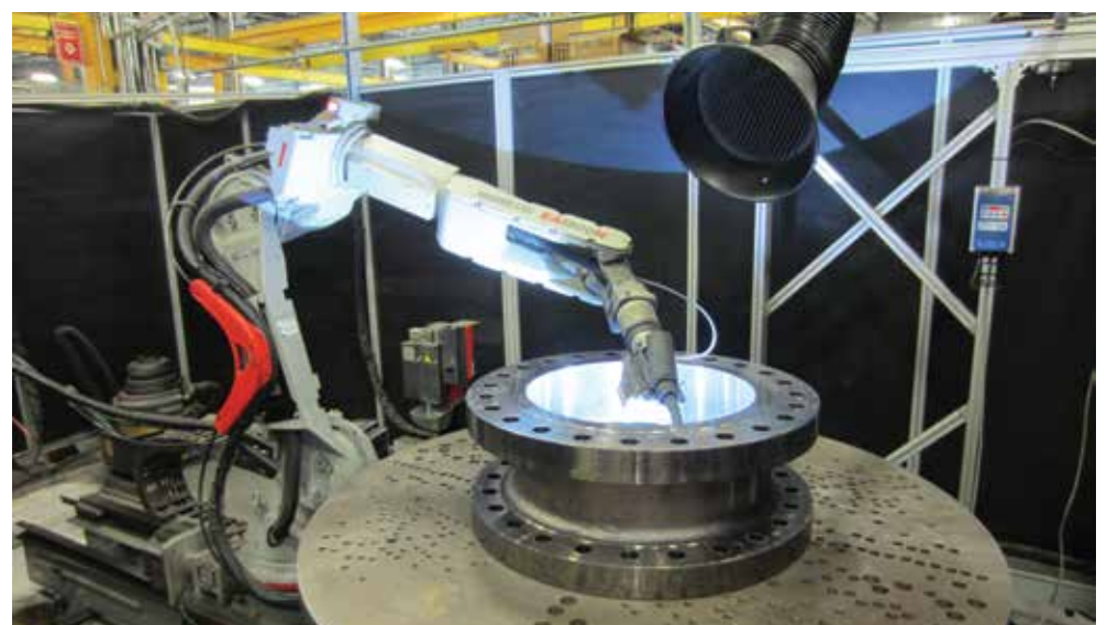
Robotic hardfacing of a dual-plate check valve.
