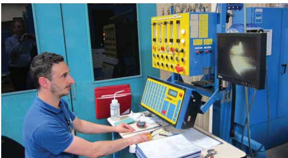
An automated welding unit in Velan's French plant, where the operator sets the parameters and then views the hardfacing operations on a screen.
