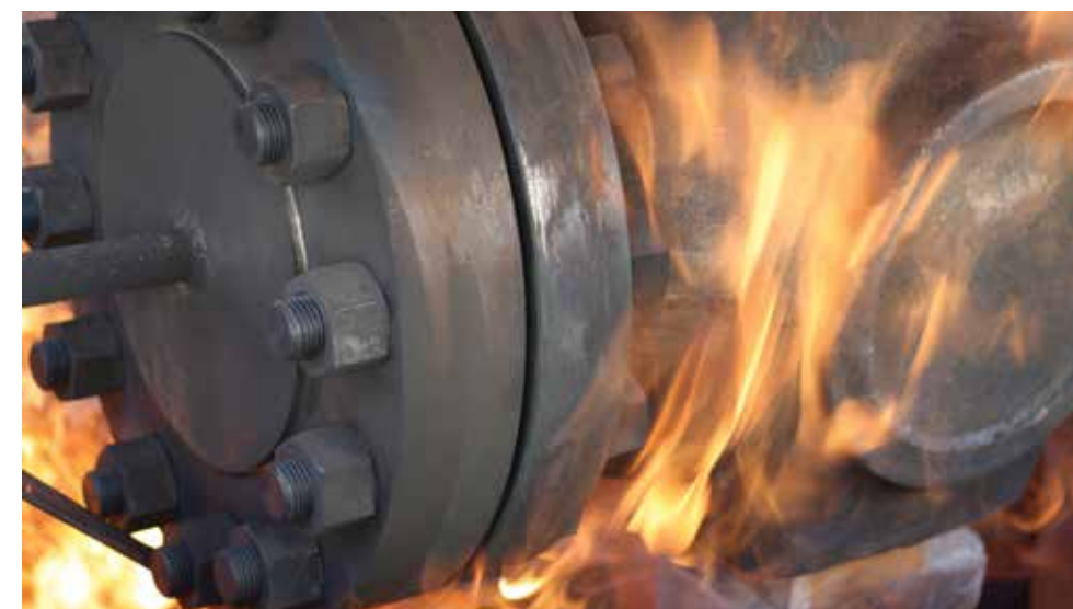
Neway valve undergoing fire test to provide maximum safety and protection for end users
