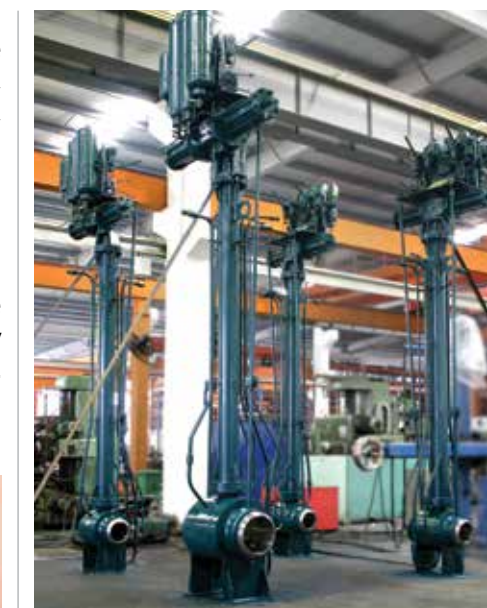
Underground ball valves with gas over oil actuators
