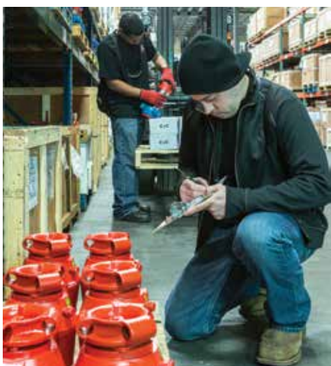
Material Supply Specialists Julio Garza & Vincent Simmons recording heat codes and serial numbers to fulfill MTR requests.
