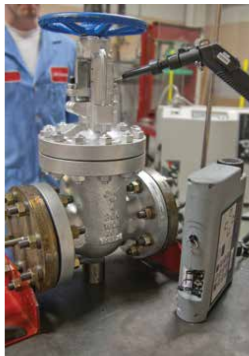
DSI confirming its Low-E packing
