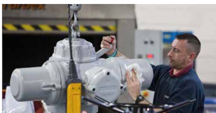
An IQ range actuator with an intumescent fire-protective coating in the final stage of assembly.
