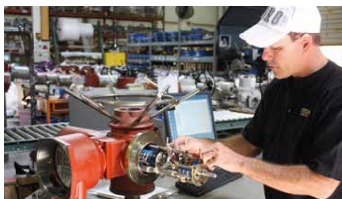
A technician tests an NA range actuator designed for nuclear power plant applications.
