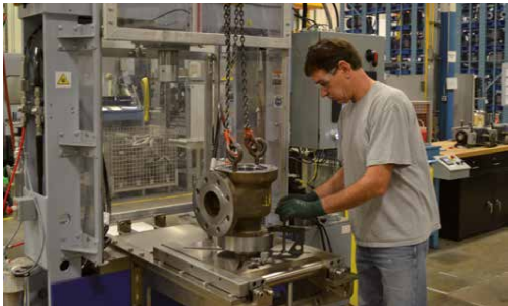
Ergonomically Designed Hydrostatic Testing Station (LEAN investment).
