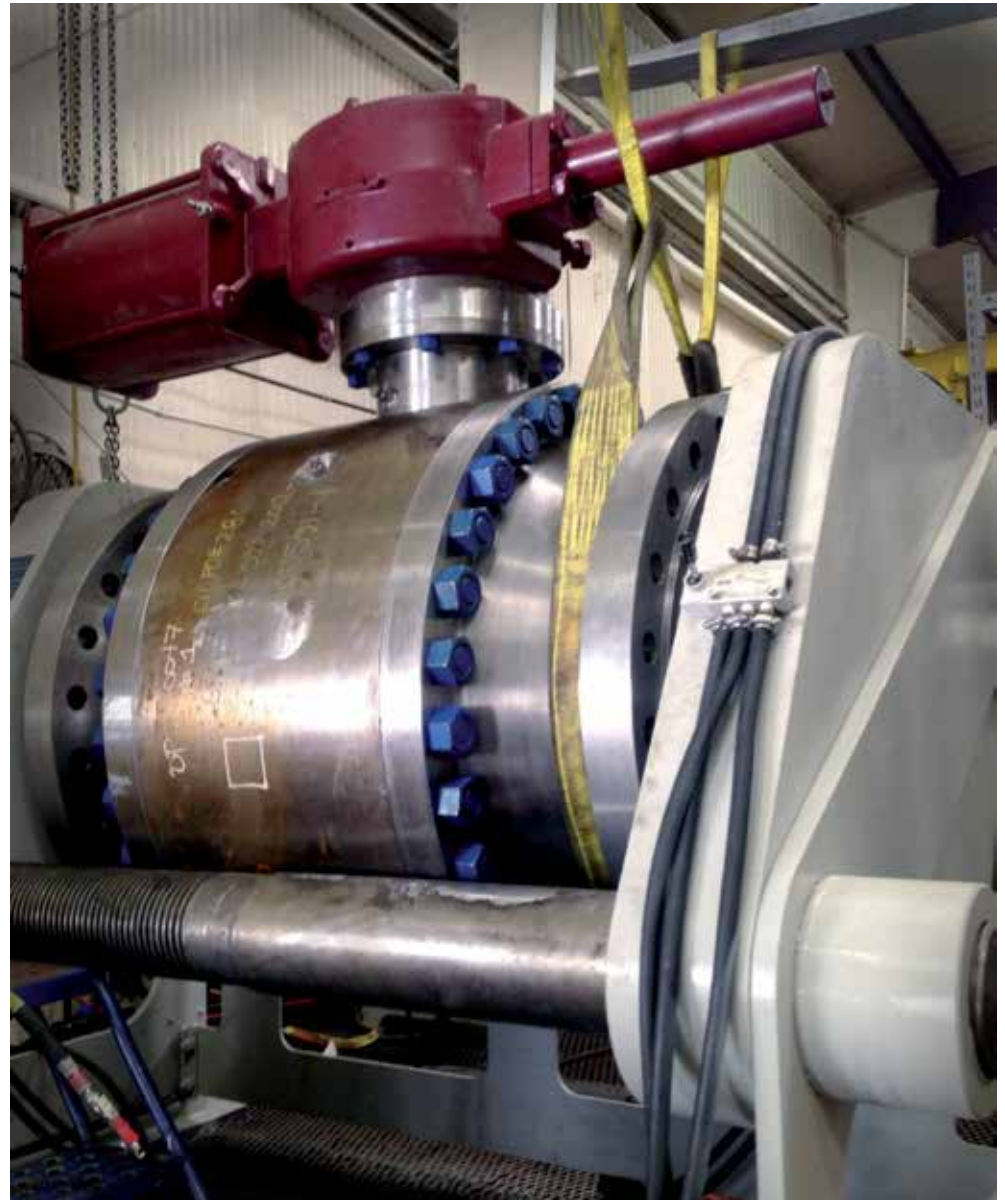
Performs API 6A, API 6D, and API 598 - Shell, seat & air testing of 1/2" – 24"
