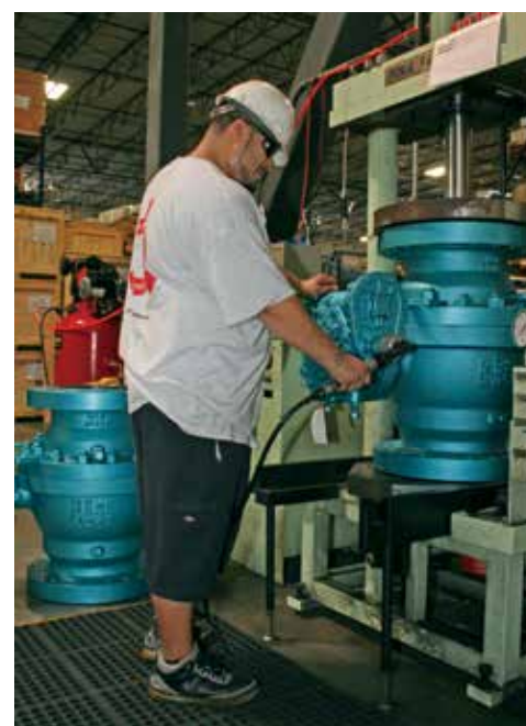
Martin Meza performs hydrostatic test on Force 8" Class 600 Ball Valve
